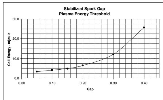
Calibration tests were run using the same test methods used for the spark plugs. The stable plasma threshold was measured with the gap set at 0.050, 0.100, 0.150, and so on. The Stabilized Spark Gap chart shows data for both positive and negative sparks, but the points lie on top of each other, so they can't be seen separately.
